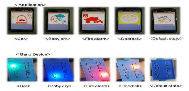
Wrist band: When you send sound results from the main device to your wristband, The LED will work for that value and the wristband will vibrate. The wrist band has one switch, which is the same as the confirmation button for the application described above.
