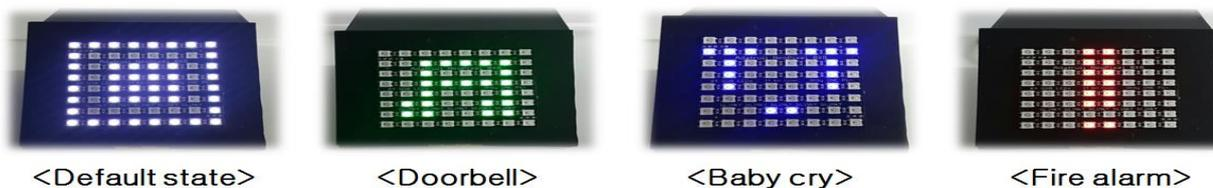
Dot matrix Display: this device is built with indoor LED lighting.
