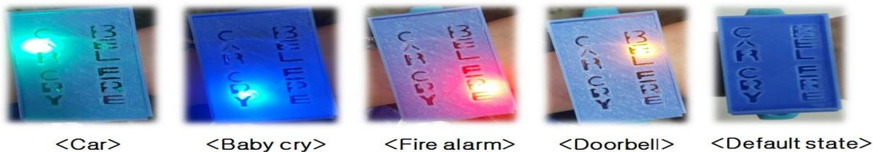
Wrist band: When you send sound results from the main device to your wristband, The LED will work for that value and the wristband will vibrate. The wrist band has one switch, which is the same as the confirmation button for the application described above.
