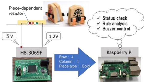
Fig.1 Concept of the proposed SHO-GI system.
